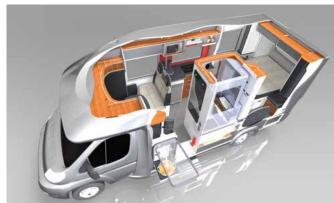
Because Trakka can use SOLIDWORKS to accurately develop its products within 3D CAD models of the luxury vans from Volkswagen, Fiat, and Mercedes-Benz that it supports, the motorhome manufacturer has virtually eliminated prototyping costs.
